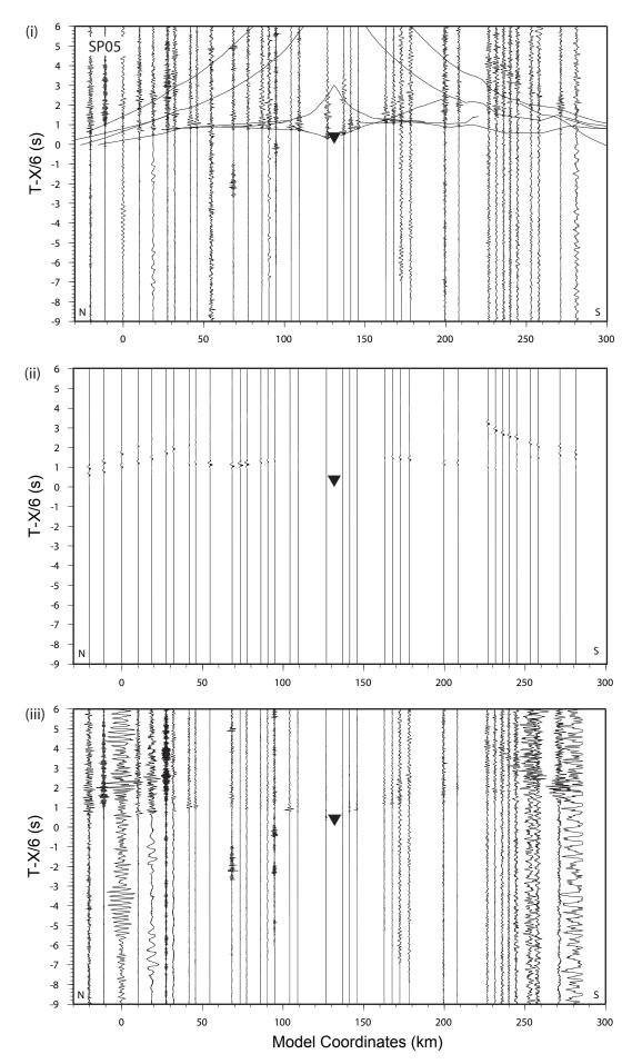
▼ shot point location; Horizontal distance in km from SP04; Reduction velocity 6 km s<sup>-1</sup> (i) Trace normalised section (bandpass filter 2-20 Hz) including picks and modelled travel-time curves for various phases derived from final model; (ii) true amplitude synthetic section derived from final model; (iii) true amplitude seismic section (bandpass filter 2-20 Hz)
